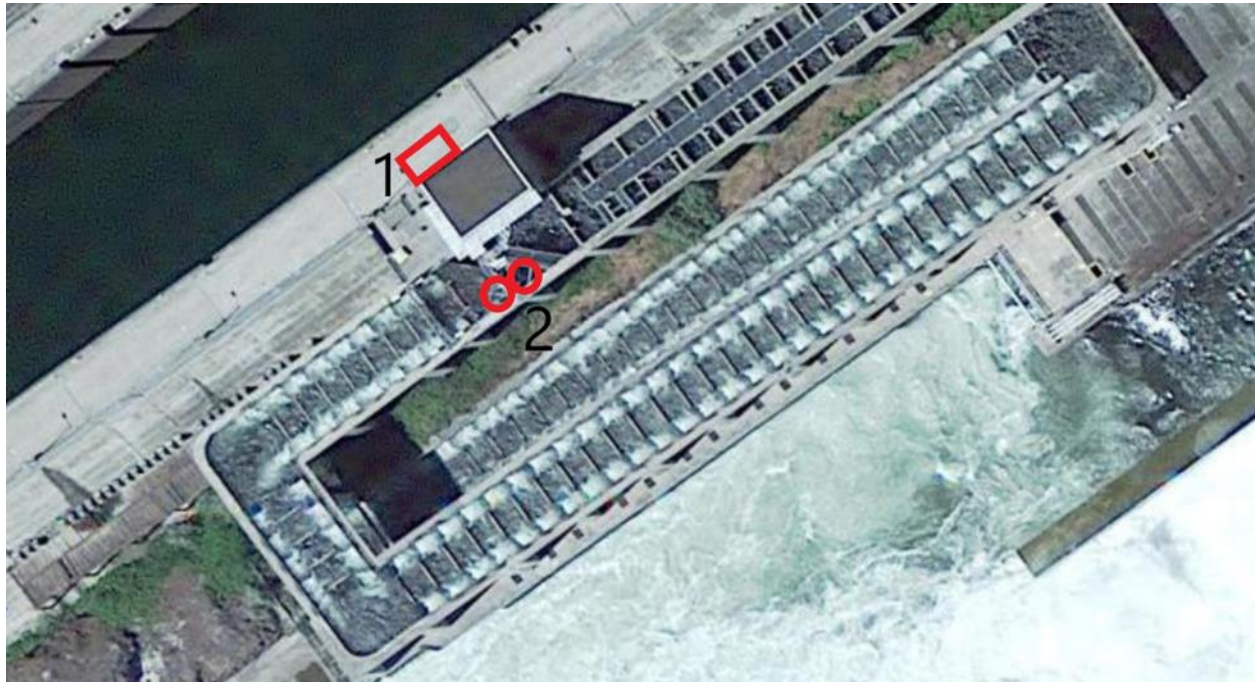
Figure 11. Close-up aerial view of the JDA North Fish Ladder. Red circles (2) denote the location of pot traps deployed above picketed leads in the fishway.
